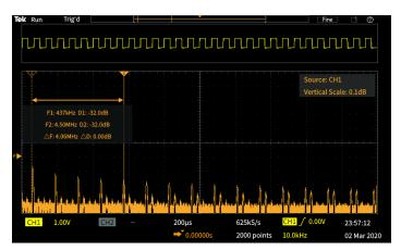
Figure 6: The time domain source waveform can be displayed above the FFT frequency spectrum
